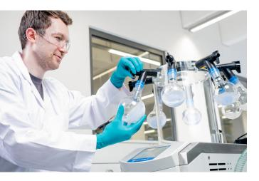
Compact, high-performance tabletop unit for effective lyophilisation of specimens in your everyday lab activities. The condenser temperature of  $-55\,^{\circ}\text{C}$  enables the drying of aqueous products.
