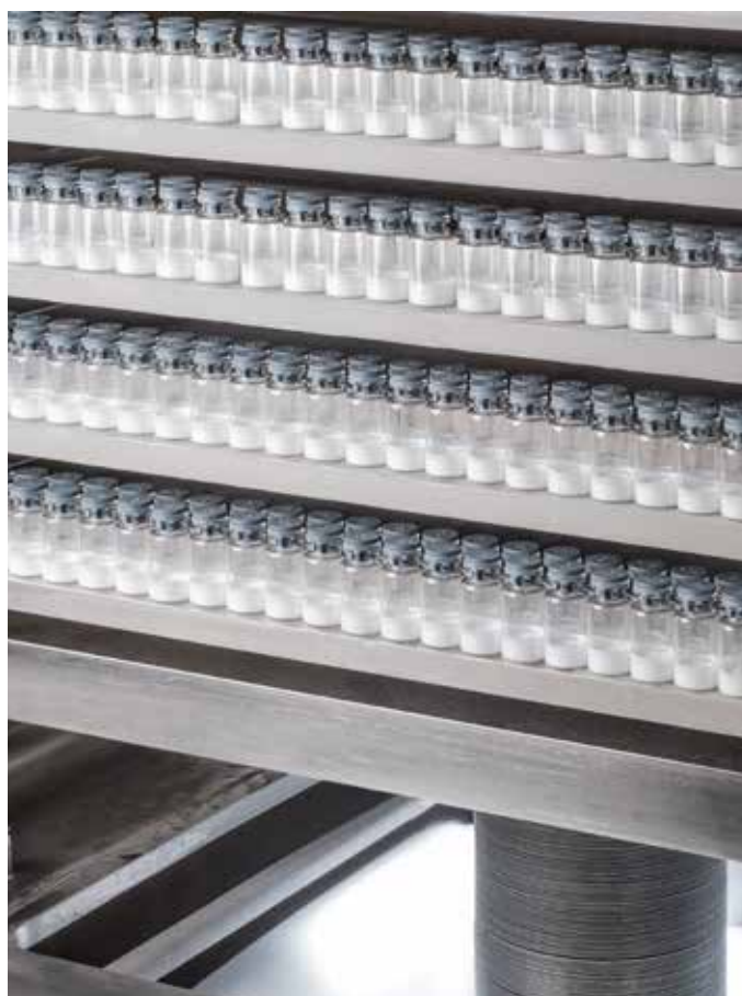
Moveable shelves for vial drying with vial closure under vacuum
