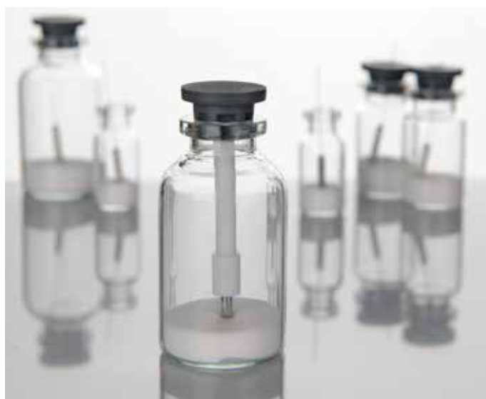
Wireless WTMplus product temperature sensors
