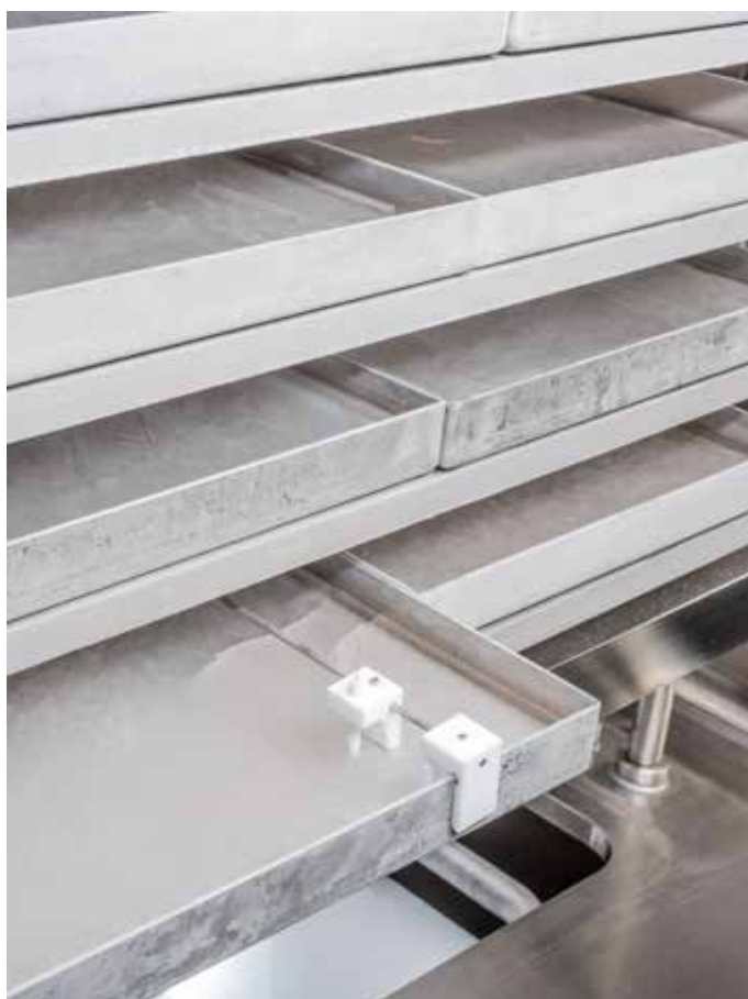
Shelves for bulk drying with fittings for the WTMplus wireless product temperature sensor
