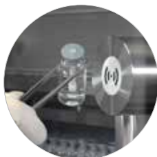
Wireless temperature measurement WTMplus 2.0 with RFID reader
