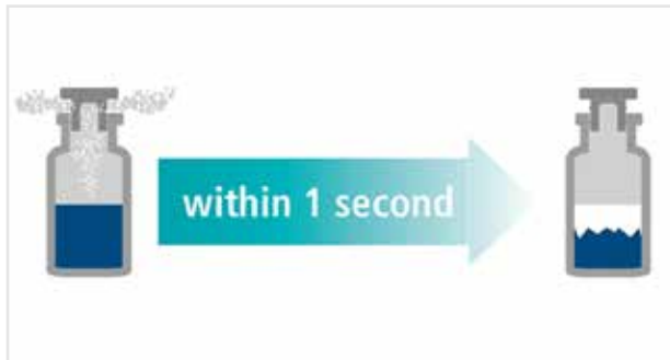
LyoCoN – controlled nucleation, ensures the simultaneous freezing of all vials
