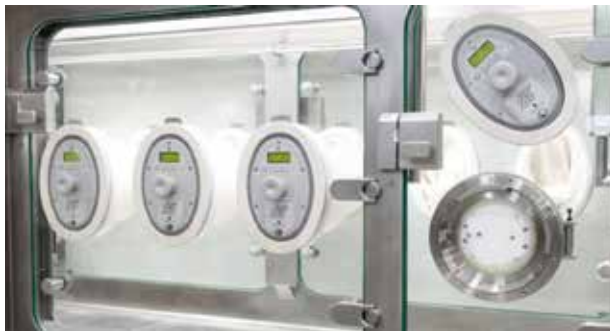
Innovative Glove Testing System for integrity testing
