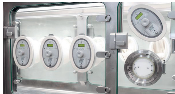
Innovative Glove Testing System for integrity testing
