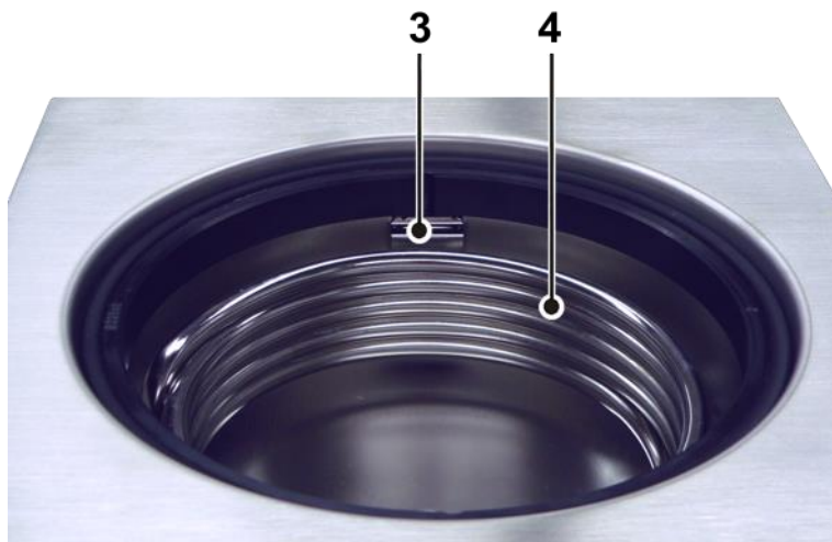
Fig. 2: Ice condenser chamber
