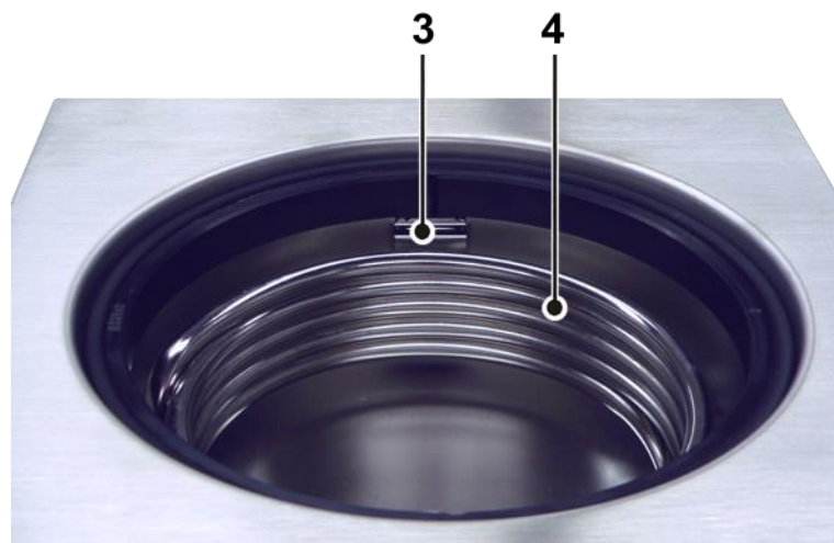
Fig. 48: Ice condenser chamber
