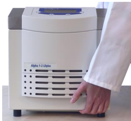
Fig. 9: Lifting the freeze-dryer
