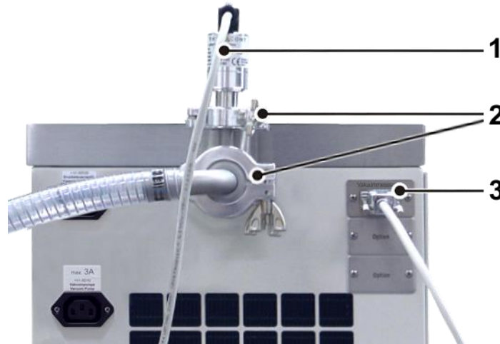
Fig. 11: Position of the vacuum sensor and the connection socket
