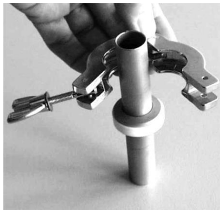
Fig. 44: Attaching the clamping ring
