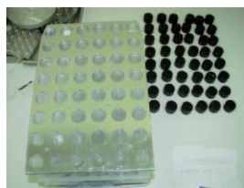
Rack with sieve cover for drying from solvent (avoidance of cross-contamination)
