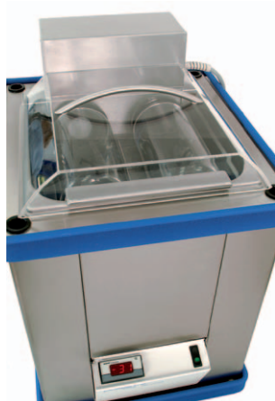
Figure 5.3 Cooling bath for freezing round-bottom flasks or wide-necked flasks under rotation (left) and drying flasks in a laboratory dryer (right)
