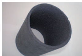
Cylinder from porous special ceramics (not a finished product)
